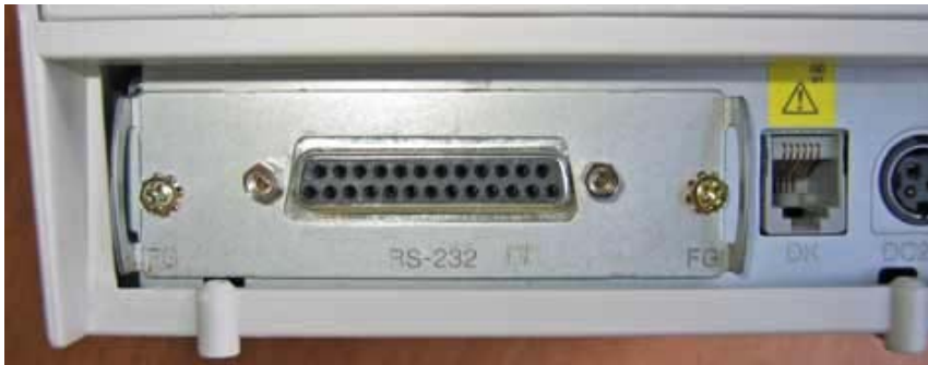
The adapter can replace the existing adapter and is held in place by 2 screws.
