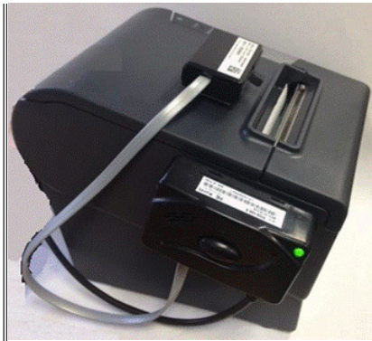
Sensor activated buzzer when paper is present
